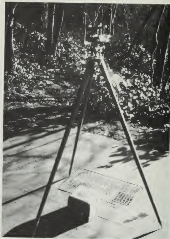
The solar compass pictured above is the type of instrument used in the original surveys of the Willamette Meridian and Base Line. The picture was taken in Willamette Stone State Park. (60)
